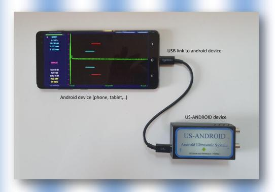
The US-Smart allows an ultrasonic control using the USB between the couple probe/US Android and your tablet or smartphone.
