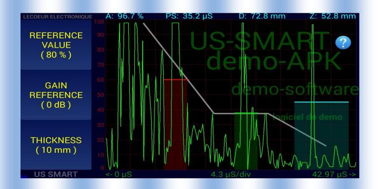
**Probe:**Allow you to set the angle of the probe, add some delay.
