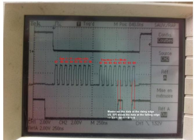
This example shows the function 9 because it needs only 1 byte DATA (0/1) and allows to ear the relay clicking when the program is ok
